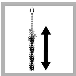
14. Clean the sample cell immediately after each test with soap, water and a brush.
