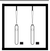
**4.** Remove the caps from 2 AmVer<sup>™</sup> Diluent Reagent High Range Test 'N Tube vials. Add 0.1 mL of deionized water to 1 vial (the blank). Add 0.1 mL of sample to the other (the
