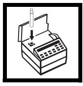
**13.** Place the prepared sample into the vial adapter with the Hach logo facing the front of the instrument. Place the cover on the adapter.
