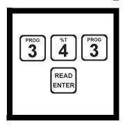
**1.** Enter the stored program for High Range Test 'N Tube<sup>TM</sup> Nitrogen, Ammonia.
