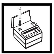
11. Place the blank into the 12. Press: **ZERO** vial adapter with the Hach logo facing the front of the instrument. Place the cover on the adapter.
