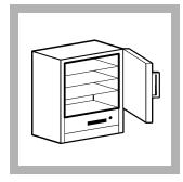
7. Place the sample in a preheated oven and evaporate at 103–105 °C (217–221 °F) for approximately 6 hours. Highly mineralized water can prolong the drying time.
