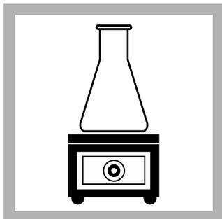
10. Put each flask on a hot plate and heat to a gentle boil.
