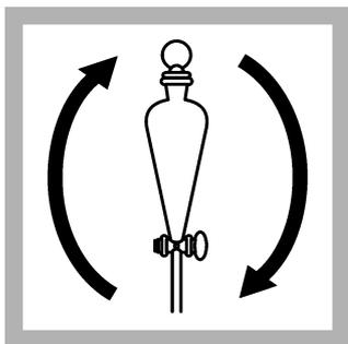
17. Swirl and invert each funnel, then open the stopcock to vent the funnel. Close the stopcock. Do this step two times with each funnel.
