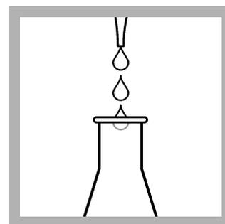
8. **For non-distilled samples:** Add 5.0 mL of Buffer Solution, sulfate type, pH 2.0 to each flask.
