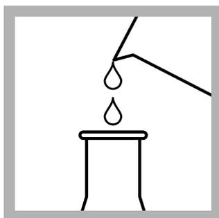
2. **Prepare the blank:** Use a graduated cylinder to add 100 mL of deionized water into a 500-mL Erlenmeyer flask. Put a mark on the flask to identify the flask as the blank.
