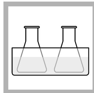
12. When the timer expires, remove both flasks from the hot plate. Decrease the temperature of the flasks to approximately 25 °C (77 °F) in a water bath.
