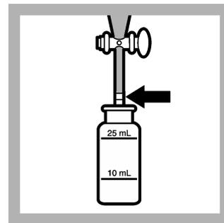
24. Insert a dry cotton plug into the outlet tube of each separatory funnel to filter the toluene and remove water or suspended particles. Identify the sample cells as blank and sample. Slowly drain the toluene from the funnels into the respective sample cells. Close the sample cells with stoppers.
