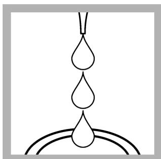
2. **Prepare the blank:** Add 2.0 mL of ammonia-free water to one AmVer™ Diluent Reagent Test 'N Tube for Low Range Ammonia Nitrogen.
