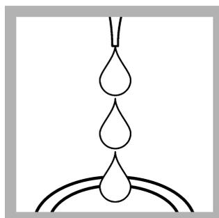
3. **Prepare the sample:** Add 2.0 mL of sample to one AmVer™ Diluent Reagent Test 'N Tube for Low Range Ammonia Nitrogen.
