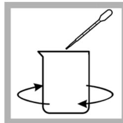
**12.** Using a 1 mL plastic dropper, add 1.0 mL of pPb-4 Neutralizer Solution to the beaker. Swirl thoroughly to mix and proceed immediately to step 13.
