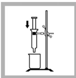
7. Soak the cotton plug with deionized water and compress it with the plunger. Remove the plunger. If the cotton plug moves up the column, push it back to the bottom with a clean, blunt rod. The cotton plug should fit snugly against the inner wall of the column.
