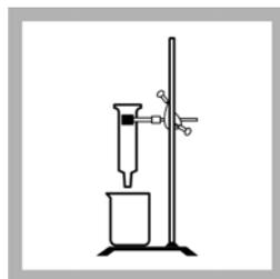
6. Mount a new Fast Column Extractor in a ring stand with a clamp. Place a 150-mL plastic beaker under the Extractor.
