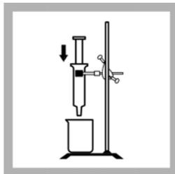
**9.** After the flow has stopped, fully compress the absorbent pad in the Extractor with the plunger. Discard the contents of the beaker. Slowly withdraw the plunger from the Extractor.
