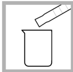
2. Fill a 100 mL plastic graduated cylinder with 100 mL of the sample. Pour the measured sample into a 250 mL plastic beaker.
