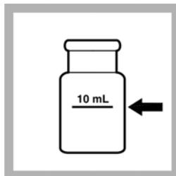
**14.** Pour 10 mL of solution into a sample cell.
