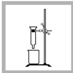
**10.** Place a clean, dry 150 mL beaker under the Extractor. Using a 25 mL plastic graduated cylinder, add 25 mL of pPb-3 Eluant Solution to the Extractor.
