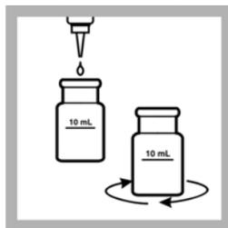
18. Remove the sample cell and add 3 drops of pPb-6 Decolorizer Solution to the cell. Swirl vigorously to mix
