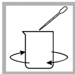
5. When the timer expires, use a second 1 mL plastic dropper to add 2.0 mL of pPb-2 Fixer Solution. Swirl to mix.
