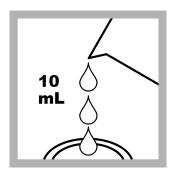
**2. Prepare the blank:** Fill the sample cell with 10 mL of sample.
