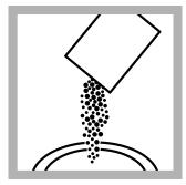
**4.** Add the contents of one Ferrous Iron Reagent Powder Pillow to the mixing cylinder.
