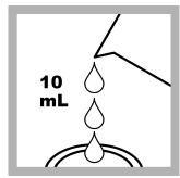
**10.** Fill a second sample cell with 10 mL of the reacted prepared sample.
