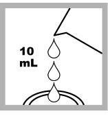
**2. Prepare the blank:** Fill the sample cell with 10 mL of sample.
