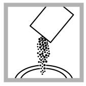
**4.** Add the contents of one Ferrous Iron Reagent Powder Pillow to the mixing cylinder. An orange color shows if ferrous iron is present in the
