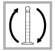
**5.** Put the stopper on the mixing cylinder. Invert the mixing cylinder several times to mix. Undissolved powder does not affect accuracy.
