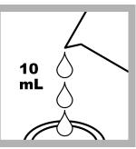
**10.** Fill a second sample cell with 10 mL of the reacted prepared sample.
