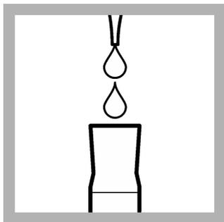
5. Use a 1.0 mL dropper to add 1.0 mL of Alkali Solution for Calcium and Magnesium Test.
