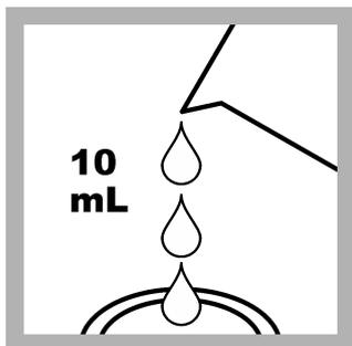
10. **Prepare the blank:** When the timer expires, fill a second sample cell with 10 mL of sample.
