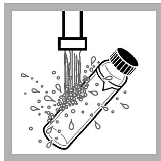
7. When the timer expires, remove the prepared sample from the water bath. Put the cap on. Use running water to cool the sample cell to 25 °C.
