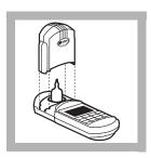
**9.** Place the AccuVac Ampul containing the sample into the instrument. Tightly cover the sample cell with the instrument cap.
