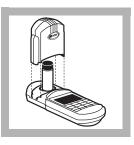
7. When the timer beeps, place the blank into the cell holder. Tightly cover the sample cell with the instrument cap.
