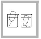
**4.** Fill a SPADNS Fluoride Reagent AccuVac Ampul with sample by breaking the tip on the bottom of the beaker. Fill a second AccuVac Ampul with deionized water (the blank).
