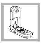
7. After the timer beeps place the blank into the cell holder. Tightly cover the ampule with the instrument cap.
