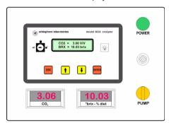
The **Power Switch** and **Pump Switch** are used to turn the instrument or pump on/off respectively.
