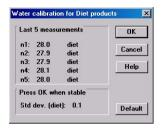
The dialog box will initially display zeros in the last five measurements column. These values are then updated every 15 seconds, as new as measurements are taken.
