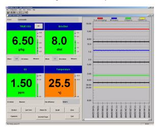
The **Numerical Indicator Panel** shows information relating to the last measurement, and is divided into four, containing the  $CO_2$  data, the Brix/Diet data, the  $O_2$  data and the temperature information. For each of these, the units of measurement, the most recent measurement value and a vertical bar graph are shown.
