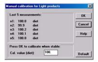
Once the measurements displayed indicate a stable condition (at least three successive stable measurement cycles), press **OK** to close the dialog box and to calculate the new slope value for the current product, which is based on the value in the edit box.
