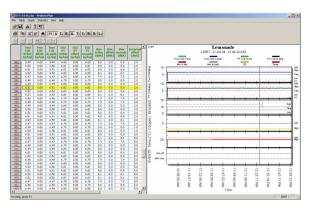
The **PBViewer Plus** program allows you to view statistical information that has been saved by the PC Program from the current or previous product runs, in a graphical and tabular format. You can start PBViewer Plus from within the ProBrix Plus PC Program by selecting **PBViewerPlus** from the **Tools** menu. This will display details for the current Product Run.
