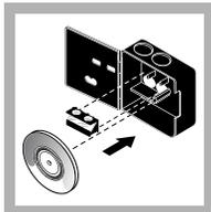
1. Install the long-path adapter in the color comparator box.
