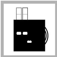
9. Put the second tube into the color comparator box.
