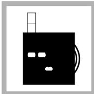
3. Put the tube into the left opening of the color comparator box.
