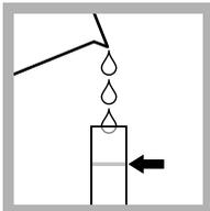
2. Fill a tube to the top line with sample.
