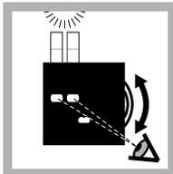
10. Hold the color comparator box below a light source. Turn the color disc to find the color match.
