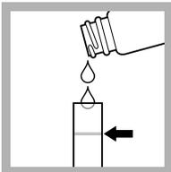
8. Fill a second tube to the top line with the prepared sample.
