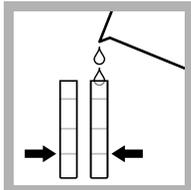
1. Fill two tubes to the first line (5 mL) with sample.
