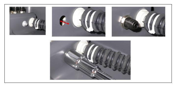
**15.** Remove the 6/4 mm PE tube as it is no longer used. Insert the red cap to avoid any leakage:
