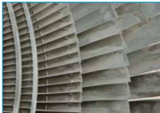
Figure 1: Silica deposition
