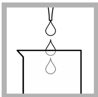
10. Add the standard solution to the beaker. Complete the remaining steps within 5 minutes.
