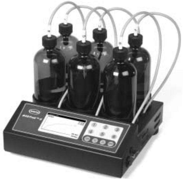
Use the Hach BODTrak II Apparatus for unattended, fast BOD (Biochemical Oxygen Demand) analysis. Features include delayed start for temperature stabilization, continuous data readout, and automatic shut-off.
