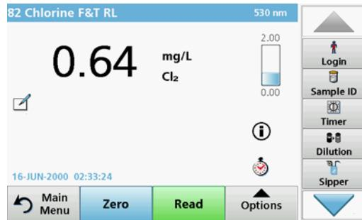
3. Place the feed tube in the sample solution and press **READ**.
