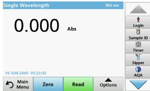
4. Place the feed tube in the sample solution and press **READ**. The sample solution is pumped in over the selected SIP time. Once the settle time has passed, the measurement is taken.
