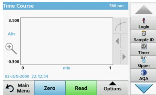
4. Place the feed tube in the sample solution and press **READ**.
