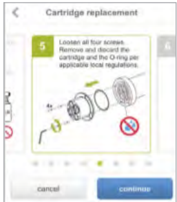
Above: Mobile Sensor Management tracks instrument status and provides step-by-step instructions to guide maintenance procedures.
