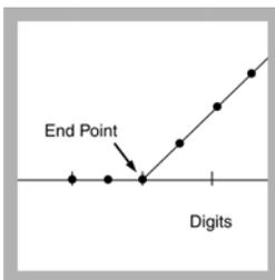
15. Determine the number of digits at the intersection of the lines. That is the standard end point.
