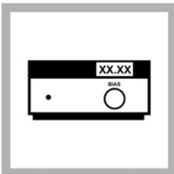
7. Note the LED reading on the Amperometric Titrator. Unlock the BIAS control knob until a stable reading between 0.50 and 0.60 is obtained. Lock the bias control.
