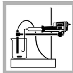
8. Using the Digital Titrator delivery knob, dispense Standard Iodine Titrant Solution in five to ten digit increments while noting the reading.
