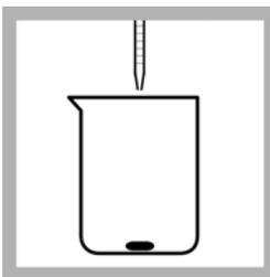
3. Place a clean, 50-mm stir bar into a clean 250-mL beaker. Use a Class A pipet to transfer 1.00 mL of 0.00564 N Sodium Thiosulfate Solution to the beaker. Alternatively, use 0.00564 N Phenylarsine Oxide (PAO) (Catalog No. 199942) instead of sodium thiosulfate.
