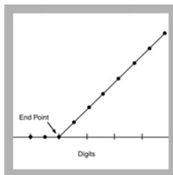
14. Draw the two best intersecting lines through the plotted points as shown above.
