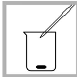
4. Use a Class A pipet to transfer 1.00 mL of 0.00564 N Sodium Thiosulfate Solution to the beaker. Swirl to mix.
