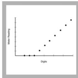
12. Using linear graph paper, plot the recorded readings from the Amperometric Titrator on the vertical axis and the corresponding Digital Titrator digits on the horizontal axis.
