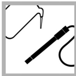
8. Remove the probe arm from the beaker and rinse the platinum wires with deionized water. Discard the sample. The adjustment of the electrode response slope is complete.
