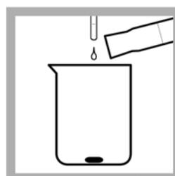
4. Add 1 mL of pH 4 Acetate Buffer Solution to the beaker. Then add 200 mL of the sample to the beaker. Minimize agitation when adding the sample. Swirl to mix.
