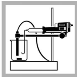
9. Continue dispensing titrant in five to ten digit increments while noting the reading.
