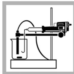
8. Using the Digital Titrator delivery knob, dispense 100 digits of Standard Iodine Titrant Solution and note the reading.
