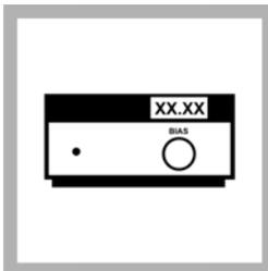
7. Note the LED reading on the Amperometric Titrator. It should read  $0.00 \pm 0.05$ . **DO NOT** adjust the bias control.
