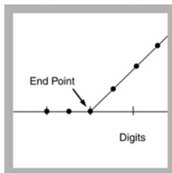
14. Determine the number of digits at the intersection of the lines. That is the sample end point.
