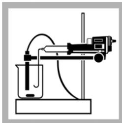
6. Place the beaker on the TitraStir stand and immerse the tips of both the probe and the delivery tube in the solution. The probe's platinum wires must be submerged. Turn on the stirring motor.
