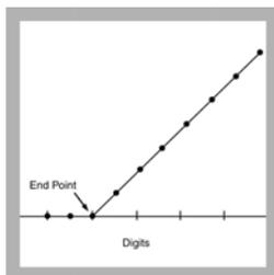
13. Draw the two best intersecting lines through the plotted points as shown above.
