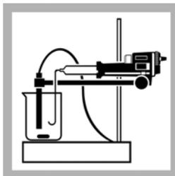
6. Use the Digital Titrator delivery knob to add 50 digits of Standard Iodine Titrant Solution.
