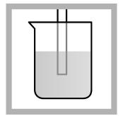
2. Laboratory test: Put the probe in a beaker that contains the solution. Do not let the probe touch the stir bar, bottom or sides of the container. Remove the air bubbles from under the probe tip. Stir the sample at a slow to moderate rate.
