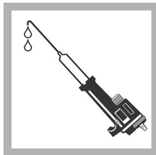
**11.** Hold the Digital Titrator vertically with the cartridge tip up. Turn the delivery tube knob to eject air and a few drops of titrant. Reset the counter to zero and clean the tip.
