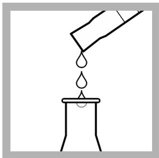
**9.** Accurately measure 20 mL of the prepared sample and transfer it to a 50-mL Erlenmeyer flask.
