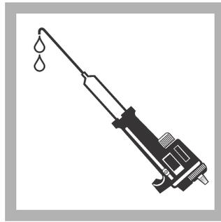
**11.** Hold the Digital Titrator vertically with the cartridge tip up. Turn the delivery knob to eject air and a few drops of titrant. Reset the counter to zero and clean the tip.
