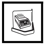
**10.** Cap the vial assemblies tightly and place them in the COD reactor for 2 hours at 103–105 °C.
