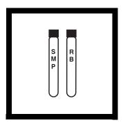
**5.** Label two Low Range Acid Digestion vials: sample and reagent blank.
