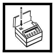
17. Place the reagent blank vial assembly into the cell holder. Close the light shield.
