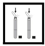
9. Lower one unopened ampule into each Acid Digestion vial. When the score mark on the ampule is level with the top of the Acid Digestion vial, snap the top off the ampule and allow it to drop into the Acid Digestion vial.
