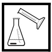
**2.** Use a graduated cylinder to add 10 mL of sample to a 50-mL Erlenmeyer flask containing a stir bar.
