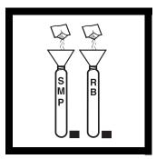
**6.** Using a funnel, add the contents of one TOC Persulfate Powder Pillow to each Acid Digestion vial (colorless liquid).
