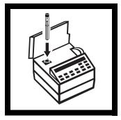
**20.** Place the sample vial holder. Close the light shield.
