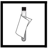
**19.** Wipe the sample vial assembly with a damp towel, assembly into the cell followed by a dry one, to remove fingerprints or other marks.
