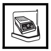
**1.** Turn on the COD reactor. Heat to 103-105 °C. Place the plastic shield in front of the reactor.
