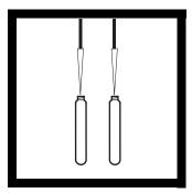
7. Use a TenSette® Pipet to 8. Rinse two blue Indicator add 3.0 mL of organic-free water to the reagent blank vial and 3.0 mL of **prepared** sample to the sample vial. Swirl to mix.
