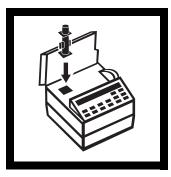
**12.** Place the COD Vial Adapter into the cell holder with the marker to the right.
