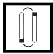
**10.** Cap and invert at least 10 times to dissolve the powder (the prepared sample).
