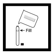
5. Fill an empty Test 'N Tube vial with sample. This is the sample blank.
