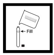
**9.** Remove the cap from a Free Chlorine DPD-TNT tube. Add 10 mL of sample.
