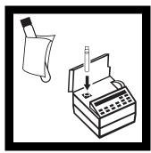
11. Within 30 seconds after 12. Press: READ/ENTER mixing, wipe the vial containing the prepared sample. Place it in the adapter with the Hach logo facing the front of the instrument. Place the cover on the adapter.
