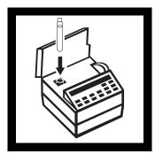
7. Place the sample blank into the vial adapter with the Hach logo facing the front of the instrument. Place the cover on the adapter.
