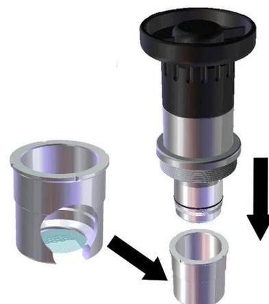
**20.** Push the protection cap firmly into place, making sure one of the four slots in the protection cap fits over the small locking pin (highlighted right). If it is necessary to turn the protection cap to fit over the locking pin, ensure you only turn it **clockwise** to avoid unscrewing the cartridge.
