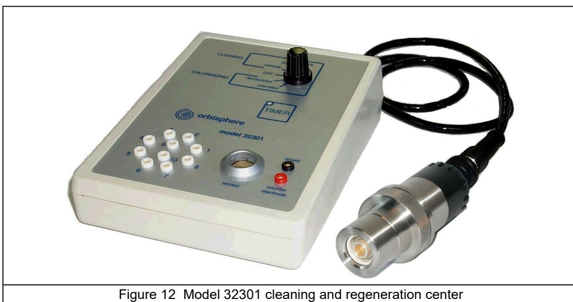
Use of this tool is recommended for a noticeably extended sensor life. Detailed information on how to use the cleaning and regeneration center is included in the 32301 Operator Manual.
