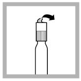
2. Carefully remove the foil from the screwed-on **DosiCap Zip A**.
