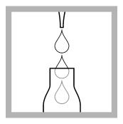
**11.** Pipet into the cooled vial: **0.2 mL** of reagent **B**. Close reagent **B** immediately after use.
