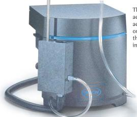
The patented modular sample compartment accommodates a variety of innovative accessories. Modules and cell holders swap out in seconds without having to turn off the DR/4000. See page 12 for more information about module configurations.
