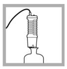
**10.** Place the LBOD Probe in the BOD Bottle containing the sample.
