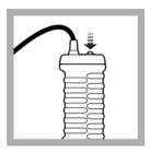
11. Engage the stir paddle on the LBOD probe by pushing the button on the top of the probe. The green indicator light on the top of the probe will illuminate when the stirrer is running.
