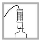
8. Probe calibration is required before initial and final BOD readings. Refer to the *Calibration* section of this procedure.
