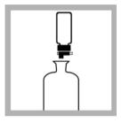
5. If the test is for CBOD, add two portions of Nitrification Inhibitor (approximately 0.16 g) to each bottle.
