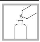
4. Fill an additional BOD bottle with dilution water only. This will be the dilution water blank.
