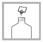
1. Prepare the dilution water using a BOD Nutrient Buffer Pillow. See Dilution water preparation.
