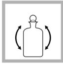
Stopper the bottles carefully to prevent air bubbles from becoming trapped. Press down on the stopper and invert the bottles several times to mix.
