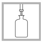
Fill each bottle to just below the lip with dilution water. Allow the dilution water to flow down the sides of the bottle to prevent air bubbles from becoming trapped in the bottle.
