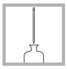
Stir the sample gently with the pipet. Use the pipet to add the minimum sample volume to the first BOD bottle.
