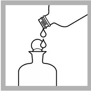
**9.** Carefully insert a stopper in each of the prepared sample bottles to prevent trapped air bubbles. Add dilution water above the stopper of the BOD bottles to make a water seal.
