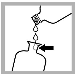
5. Fill each bottle with prepared dilution water. Refer to [Prepare the dilution water](#) on page 3. To prevent air bubbles, pour the water down the inner surface of the bottle.
