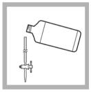
2. Fill the buret to the zero mark with 0.0125 N Potassium lodide-lodate Standard Solution.
