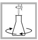
6. Titrate the sample while gently swirling the flask until the color changes to a permanent blue color (end point).
