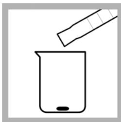
2. Put a 50-mm stir bar into a 250-mL beaker. Use a graduated cylinder to measure 200 mL of sample. Add the sample to the beaker.
