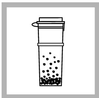
6. Let the particles settle for a minimum of 1 minute. Carefully open the extraction vial.
