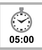
**6.** Start the instrument timer. A 5-minute reaction time starts. An amber color shows if nitrate is present.
