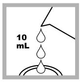
**7. Prepare the blank:** Fill a second sample cell with 10 mL of sample.
