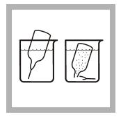
3. Prepare the sample: Collect at least 40 mL of sample in a 50-mL beaker. Fill the AccuVac Ampul with sample. Keep the tip immersed while the Ampul fills completely.
