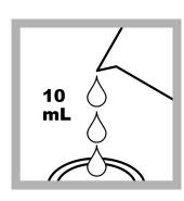
**6. Prepare the blank:** Fill a sample cell with 10 mL of deionized water.
