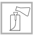
**12.** Pour the contents of the flask containing the prepared sample into the Pour-Thru Cell.
