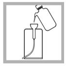
**2.** Flush the Pour-Thru Cell with 50 mL of deionized water.
