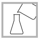
3. Rinse two clean 125 mL Erlenmeyer flasks with the sample three times.
