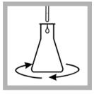
7. Prepared sample: Add 1.0 mL of FerroZine Iron Reagent Solution to flask using the Dispenser. Swirl to mix.
