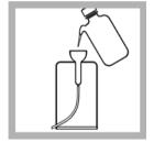
**14.** Flush the Pour-Thru Cell with at least 50 mL of deionized water immediately after use.
