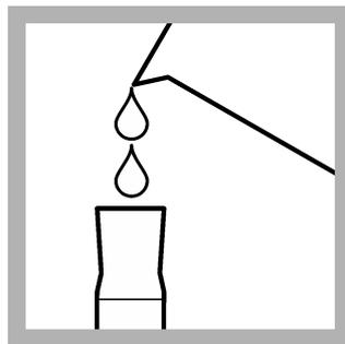
7. Carefully fill the mixing cylinder to the 80-mL mark with sample.
