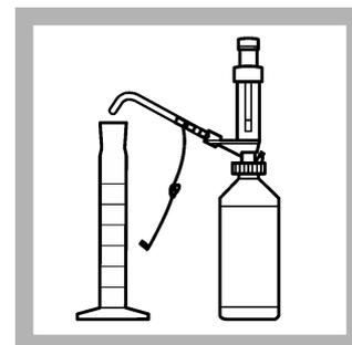
4. Use the bottle-top dispenser to add 1.0 mL of Free Chlorine Buffer Solution to a clean, dry 100-mL glass mixing cylinder.
