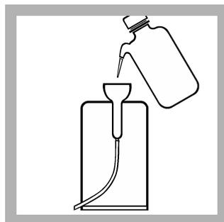
11. Flush the Pour-Thru Cell with at least 50-mL of deionized water immediately after use.
