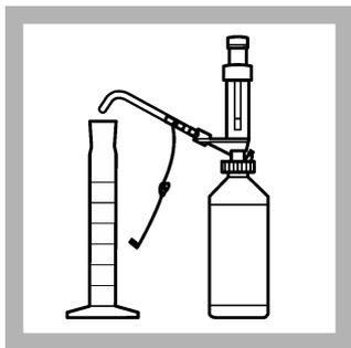
5. Use the bottle-top dispenser to add 1.0 mL of prepared Free Chlorine Indicator Solution to the same mixing cylinder.
