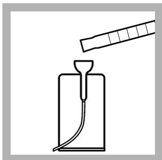
9. Fill the funnel of the Pour-Thru Cell with the reacted sample from the mixing cylinder. It is not necessary to pour all of the sample into the Pour-Thru Cell; approximately half of the sample can be discarded.
