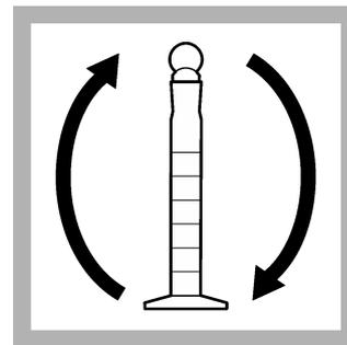
8. Put the stopper on the mixing cylinder. Lightly invert twice to mix. Continue immediately to the next step.
