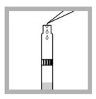
2. Carefully pipet 2.0 mL of sample into the vial. Immediately proceed to step 3.
