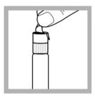
1. Carefully remove the protective foil lid from the DosiCap<sup>TM</sup> *Zip*. Unscrew the cap from the vial.
