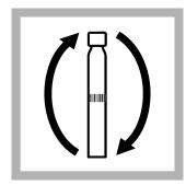
4. Tighten the cap on the vial and invert until completely mixed.
