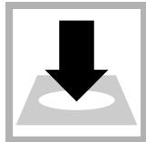
7. Insert the Zero vial into the cell holder. DR 1900 only: Push ZERO. The instrument zero is set.
