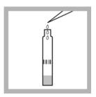
1. Pipet 2.0 mL of Solution A into the vial.
