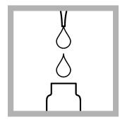
1. Use a pipet to add 2.0 mL of Solution A to the test vial.
