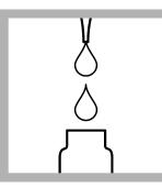
2. Use a pipet to add 3.0 mL of sample to the test vial.
