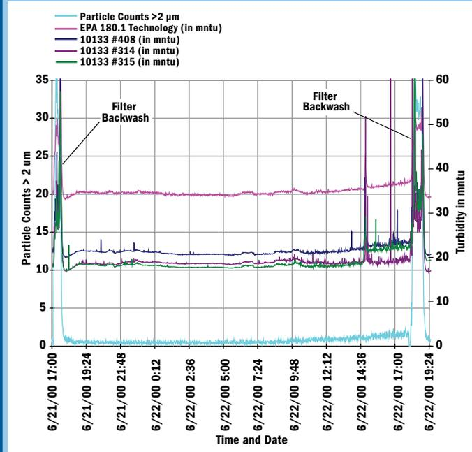
laser turbidity readings can provide a qualitative assessment regarding the nature of membrane integrity loss.
