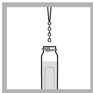
3. Use a sterile pipet to transfer 10 mL of sample into each of the 10 tubes of Lauryl Tryptose broth. Do not touch the open end of the tubes or the inner surface of the caps. Immediately replace and tighten the screw cap on each tube.
