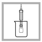
2. Laboratory tests: Immerse the probe in a beaker containing the sample solution. Move the probe up and down and tap it on the beaker to remove bubbles from the electrode.
