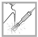
4. Rinse the probe thoroughly with deionized water after each measurement.
