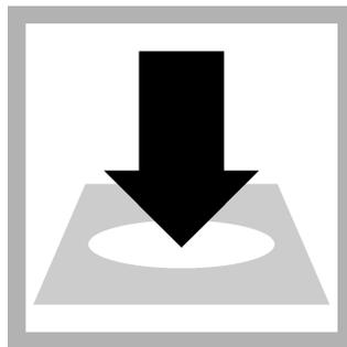
11. Within 3 minutes after the timer expires, insert the prepared sample into the cell holder.
